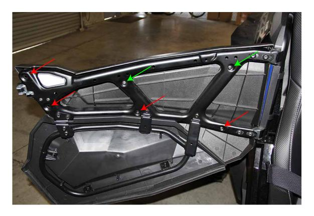
**STEP #2**Attach the supplied Velcro mounting strip to the door frame using the 3 factory screws indicated below.
